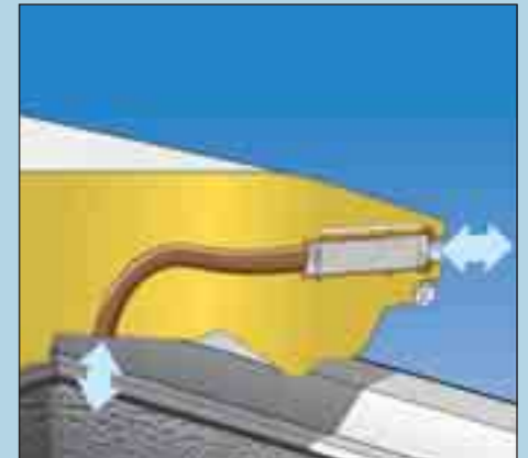
StopFrost. This innovation has two distinct advantages: frosting up of the freezer and frozen food is reduced by over 70%, reducing the number of times you need to defrost the freezer. The StopFrost system prevents a vacuum from building up after the lid has been opened and closed.
